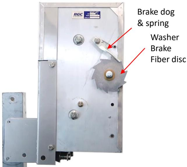
Remove the cover and then remove the brake dog, spring and the washer, brake, fiber disc. These items will no longer be used. Reinstall the cover when finished.
