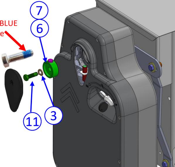
1. Install the black thick motor washer & holding bolt to secure the motor to the shaft. After tightening the back side of the motor should be tightly against the collar on the shaft.
