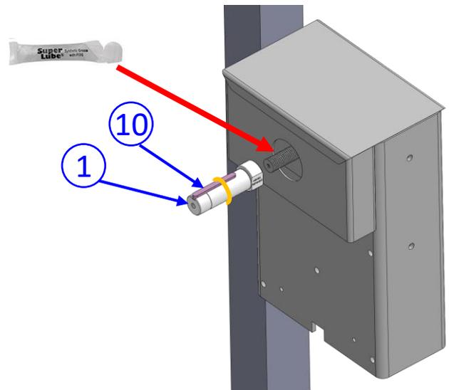
1. IMPORTANT: Grease the threaded winch shaft BEFORE installing the key adapter.
