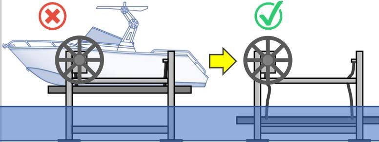
Fully lower the boat lift, remove the boat and any weight from the boat lift carriage. The cable should be slack. Ensure the lift carriage is fully down.
