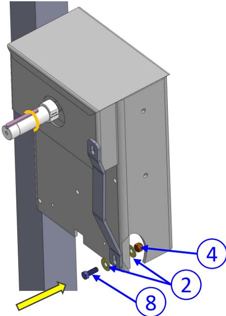
1. Attach the hold arm to the lower right corner of the winch box as shown.
