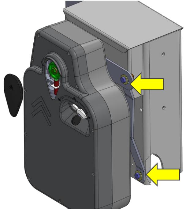
1. Make necessary adjustments to motor torque arm and hold arm positions then tighten all bolts & nuts securely.
