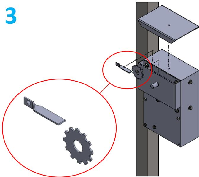
Remove the top cover and then remove the break dog and brake disc. These items will no longer be used. Reinstall the top cover when finished.
