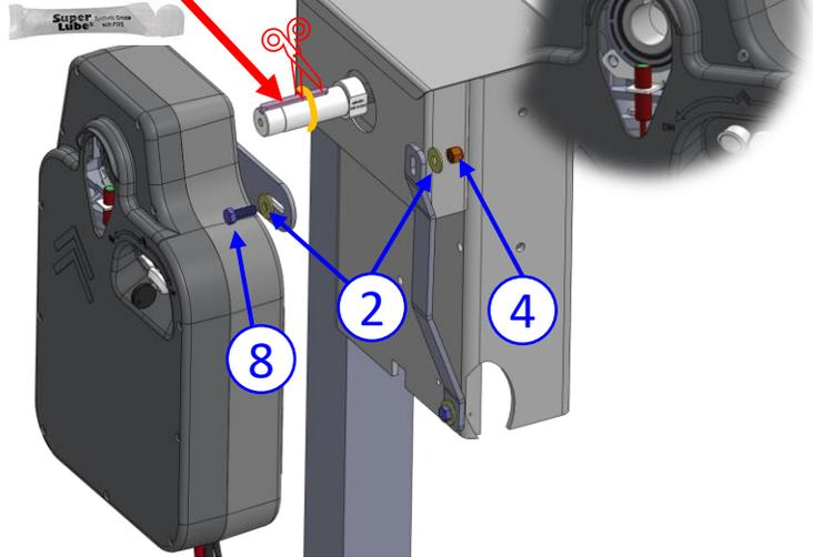
1. Grease key shaft & key before installing motor
