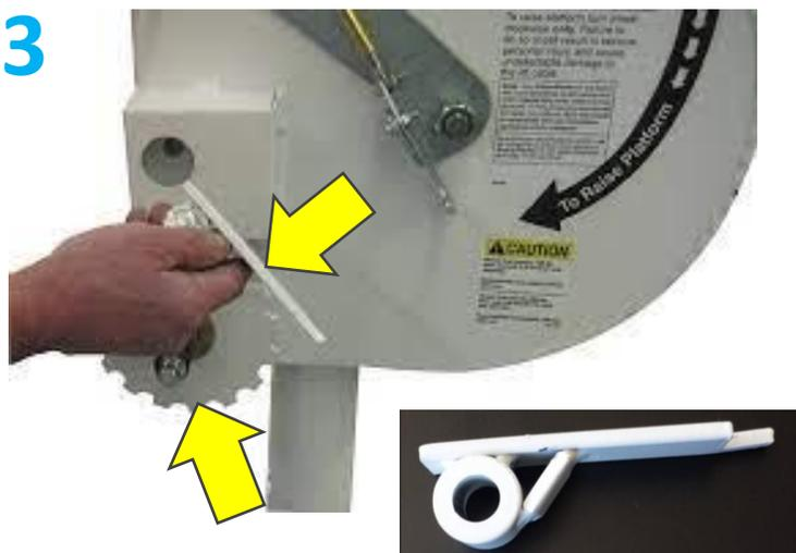
Remove the break dog and brake disc. These items will no longer be used.
