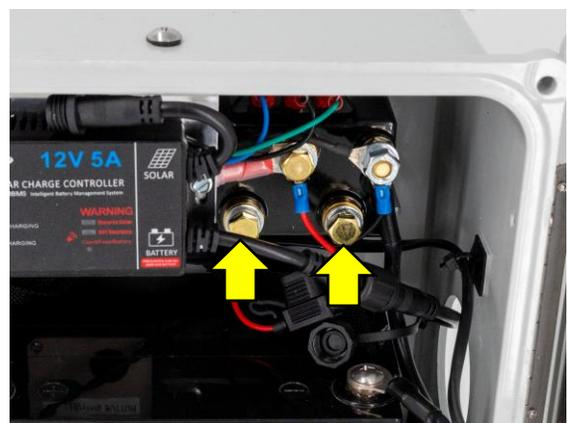
Connect the motor wires to the contactor studs labeled M1 & M2:
