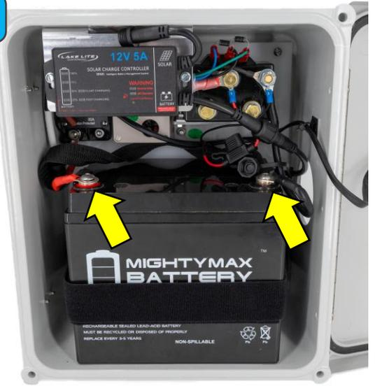
Connect the power controller cables for both motor & solar charge regulator to the battery terminals
