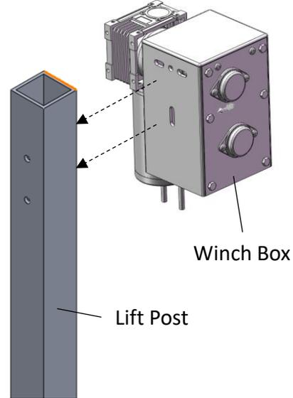
Use hardware to attach the winch box and fiberglass mount to the lift post as needed.
