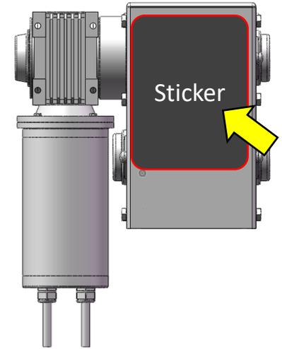
After mounting the winch to the lift, place the sticker over the exposed holes.
